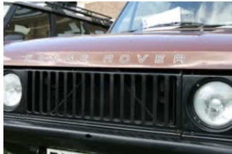
Self adhesive badges front and rear replaced the former separate plastic letters
