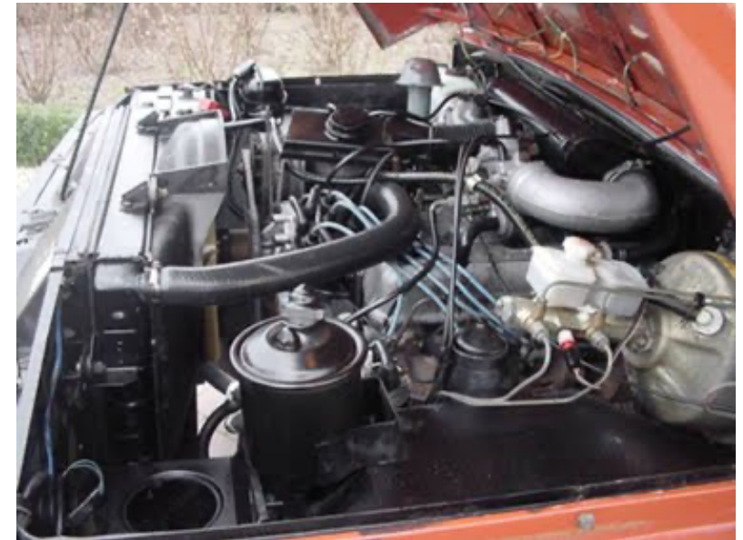
Shown is metric thread braking master pump with horizontal mount
