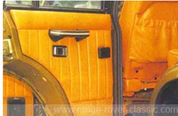
New angled heel board for easier entrance to the rear New door cards with leather, carpet and new handles Luxurious leather interior, cubby box and A/C visible
