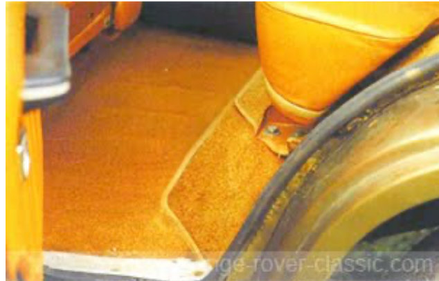
New angled heel board for easier entrance to the rear New door cards with leather, carpet and new handles Luxurious leather interior, cubby box and A/C visible
