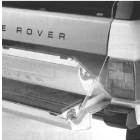
Counterbalanced tail gate by torsion bar
