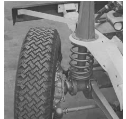
Up-rated shocks and softer rear springs
