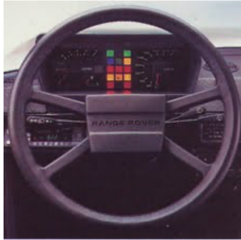
New instrument binnacle with rev counter seen
