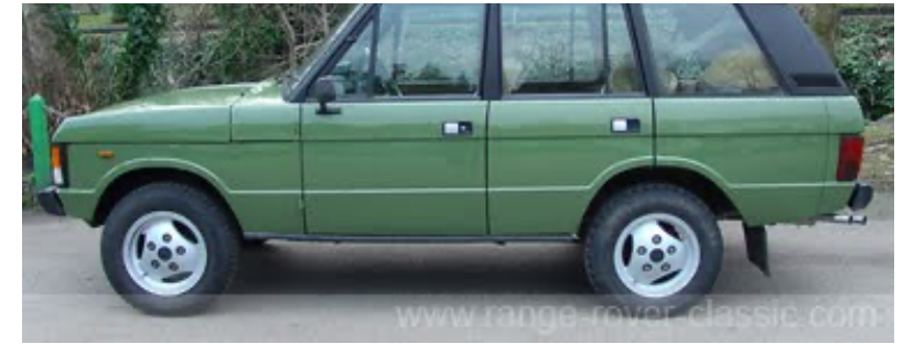
1984MY is easily recognized by the move of keyhole to door handle
