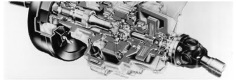
Chain Driven Transfer box with Viscous Control Unit
