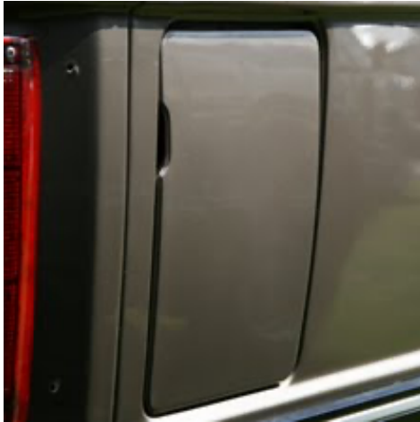
Concealed fuel filler flap on both 2D+4D
