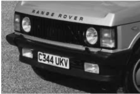
'86MY EFI Vogue: Spoiler with fog lamps, bumper wrap around end caps and body coloured lower grille area
