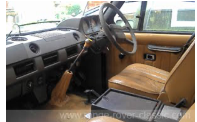
Check the new position for the ashtray on cubby box The front seats still had the handles with tilt/slide The new fascia with larger binnacle, A/C and leather
