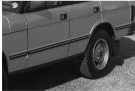
Rubber protection side strips with bright inserts replaced previous year's tape strips on Vogue model
