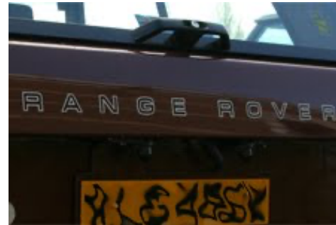
Self adhesive badges front and rear replaced the former separate plastic letters
