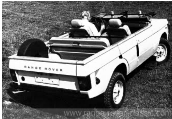
4 door fully open FLM Panelcraft conversion seen above.
