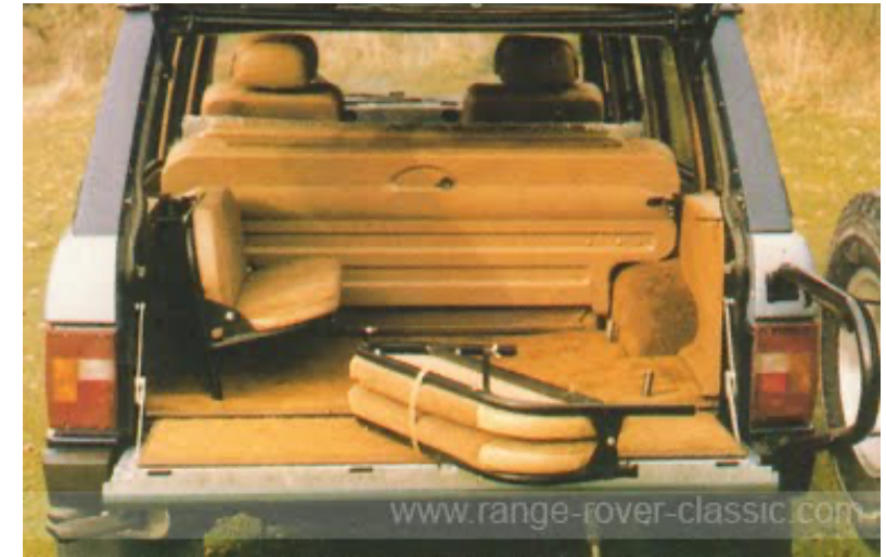
In Middle East's hot climate air conditioning front and rear are needed Here is the removeable 4-seat arrangement at rear clearly shown
