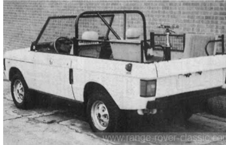
Glenframe Falcon 2-door with armoury mount for military use
