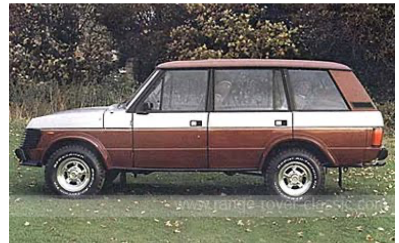
Glenframe Filton with 9" longer wheelbase and special front end
