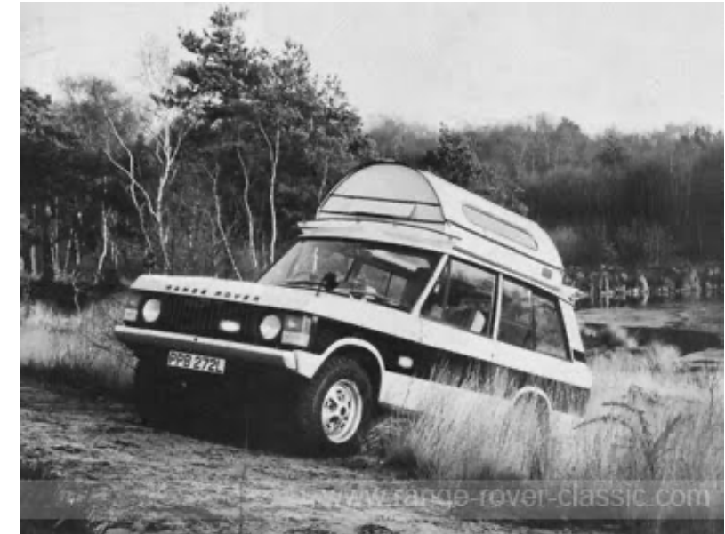
Carawagon camper conversion clearly shown here with the Searle raising roof both in lowered and raised position. Characteristic profile.
