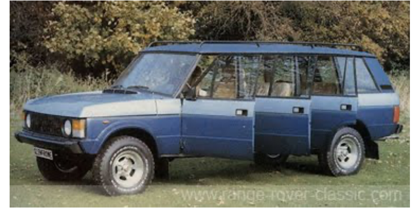
Glenframe Portway with 136" wheelbase and 6 doors
