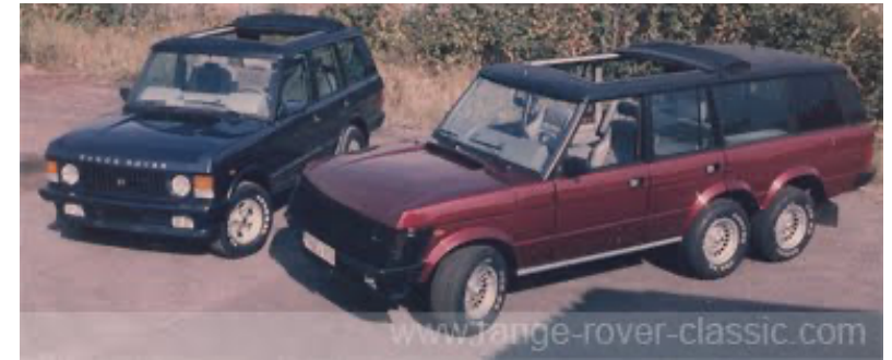
Auto Kugel, did both 3 axle and Mercedes V8 engine conversions
