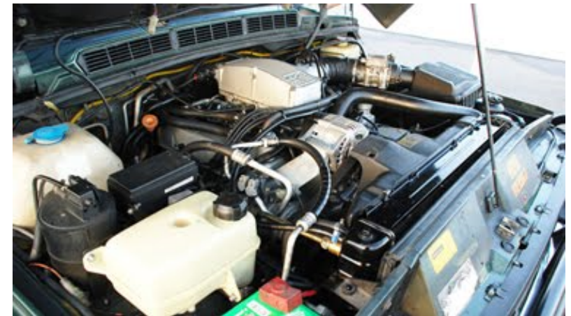
The new 4.2 ltr EFI V8 "serpentine" engine with only one pulley belt
