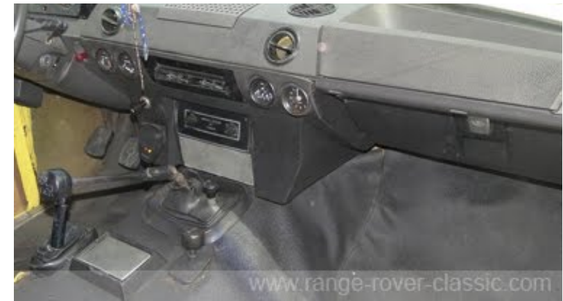
No heater, but air conditioning installed instead in Venezuela
