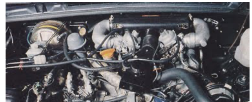
Ritter developed a 5.0 Holden Brock 184 hp performance engine kit
