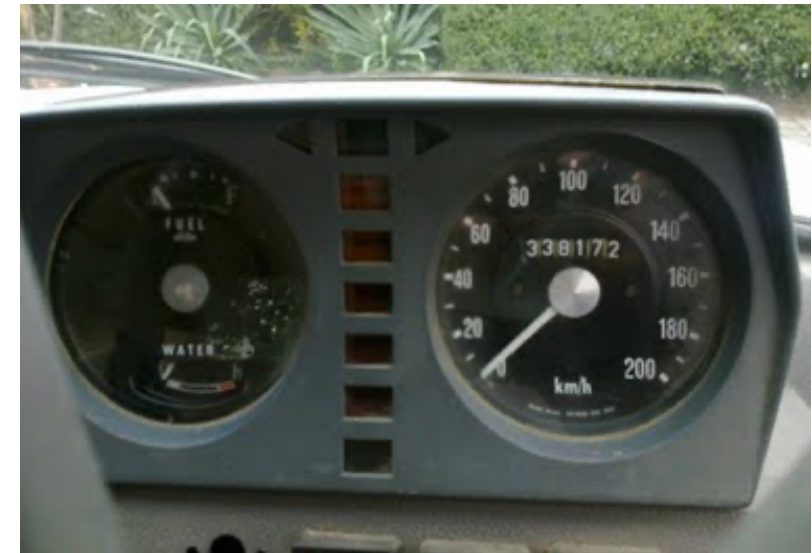
This 2 door 1984 was delivered with automatic, not available in UK Special Australian '84 binnacle with 6 digit odometer and no tripcount
