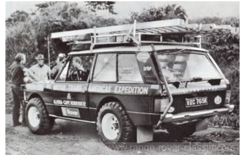
One of the Expedition Range Rovers fully equipped and fitted with extra large 'swamp' tyres. The pristine condition of the vehicle indicates that the worst was yet to come.
