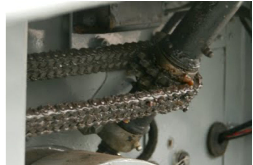
Clearly visible is the chain solution of the Centre Steering Land-Rover
