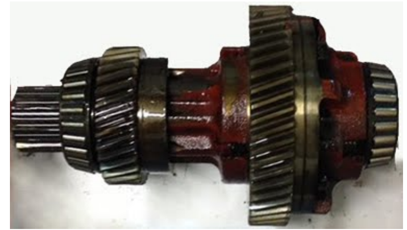
Red Salisbury differentials used in all Suffix A LT95 gearboxes - visible for the trained eye; a non-Limited Slip version
